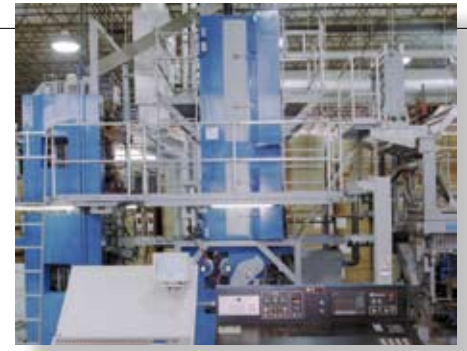
Vertical COANDA Plus Dryer for Newspaper and Commercial Printers with space restrictions
