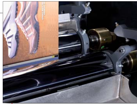
Innovative silicone applicator with cooled rollers for even and low film weights.
