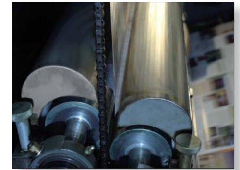
A cool bead of silicone being applied to the web by chilled applicator rollers.
