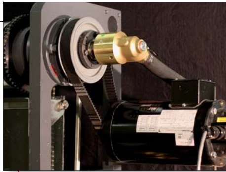
Robust steel rollers are driven, allowing use of conventional rotary unions and bearings.
