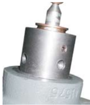
Figure 4. Setscrew location that is used to allow the plunger assembly to be removed from the plunger housing.
