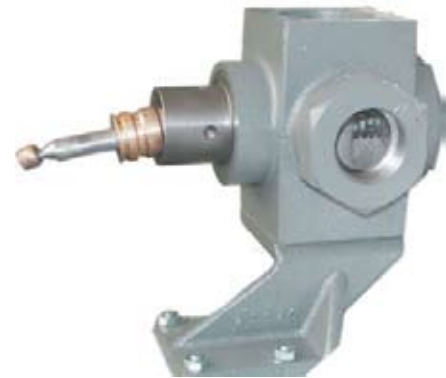
Figure 3. Plunger assembly being removed from the plunger housing. Do not pull the shaft out of the brass insert until the entire plunger assembly has been removed!
